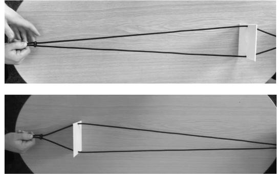
Figure 3 An initial design for a model to demonstrate the concept of angular size.
